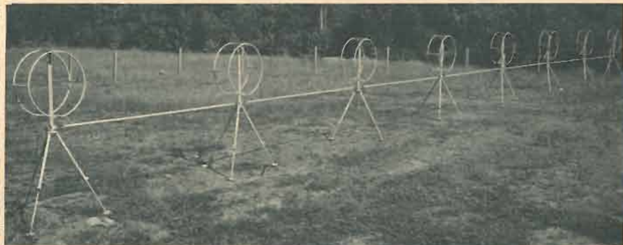
Fig. 1. Typical aperiodic loop antenna array has 36 elements in 50-meter circle.
